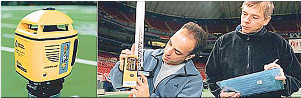
Figure 6.57 Here a laser-leveling device is used to characterize the vertical surface of the playing field. (Source: Sportvision/NY Times)
