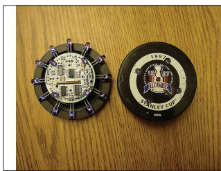
Figure 6.49 The challenges in implementing the FOX Puck effect were many, and a number of subsystems had to be designed and integrated into a single system. The first was the puck itself. Here is a "FOX" puck and its innards.
